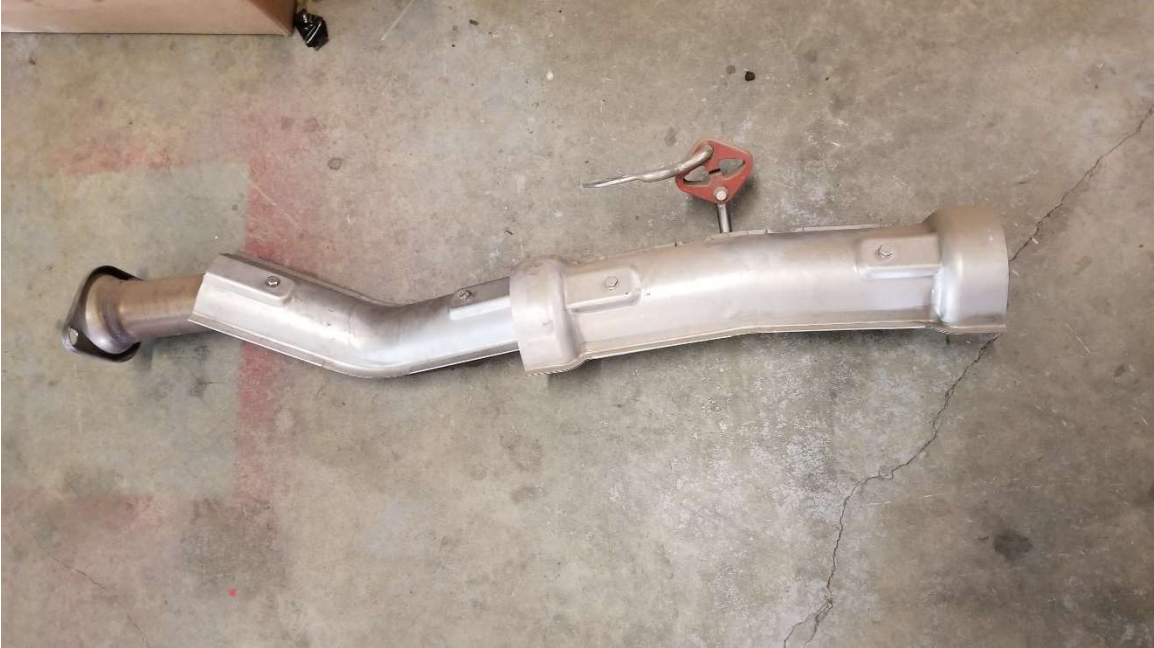
Required section to remove to get access to the transmission cooler lines entering the transmission
