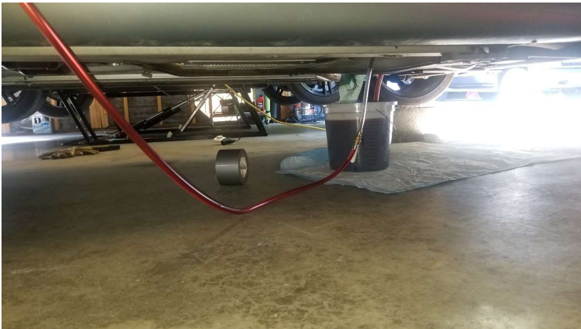
Drain bucket (8 quarts) and the new fluid going in
