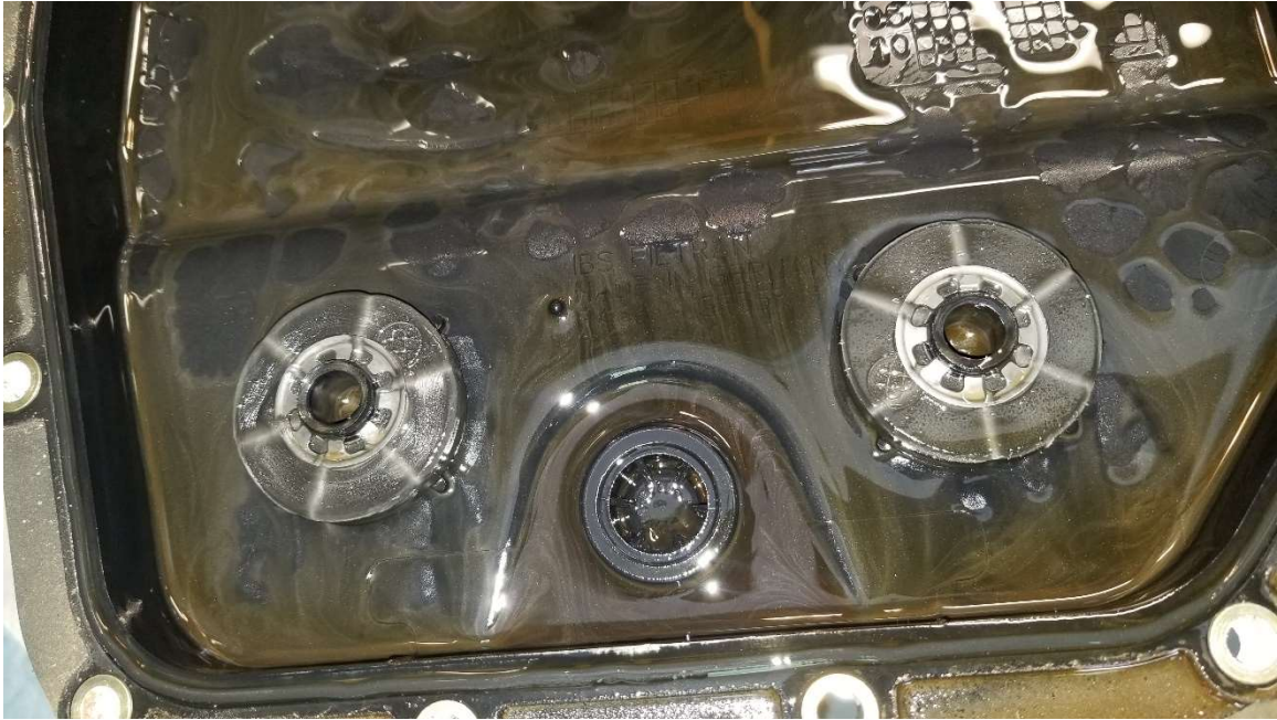
Close-up of the Pan Magnets - not a lot of debris after 15 years and 22k miles
